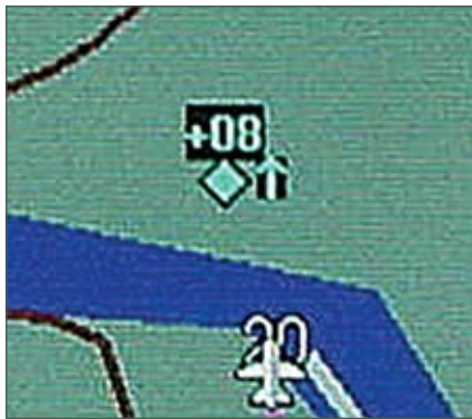
Traffic displays use standard symbology, as shown on the FlightMax EX500, above. Relative altitude data inside black boxes can be difficult to read, lower photo.
