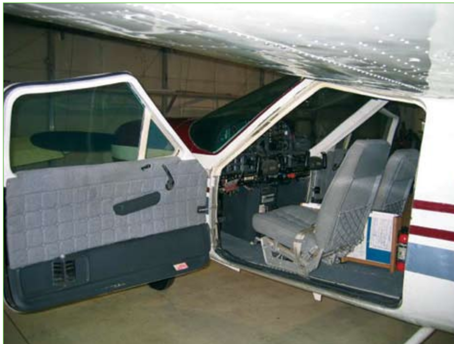
Cardinals are renowned for their barnlike cabin doors, as shown in Ken Towl's 1975 model, above. The baggage compartment is awkwardly bisected by a hump to contain the landing gear, right. Early Cardinals have a unique dip-down glareshield, as shown in the 1972 RG owned by Ross Youngblood, right.
