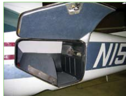
Cardinals are renowned for their barnlike cabin doors, as shown in Ken Towl's 1975 model, above. The baggage compartment is awkwardly bisected by a hump to contain the landing gear, right. Early Cardinals have a unique dip-down glareshield, as shown in the 1972 RG owned by Ross Youngblood, right.
